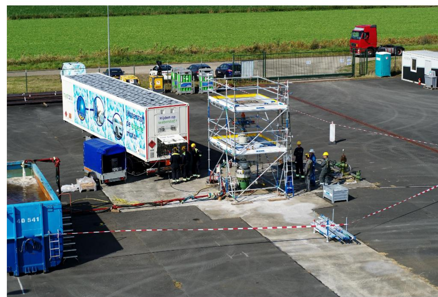
Safety testing in wells for the injection of hydrogen into underground storage (salt caverns)
